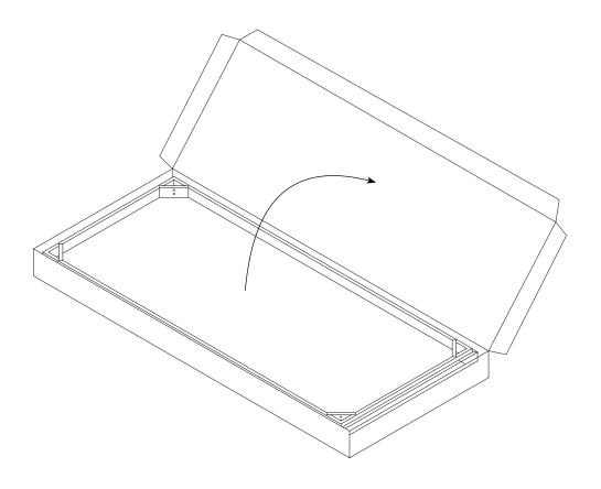
**2.** All corners are numbered 1, 2, 3 and 4. Find the corresponding leg to the corner and put in place. Insert and tighten the bolts provided.
